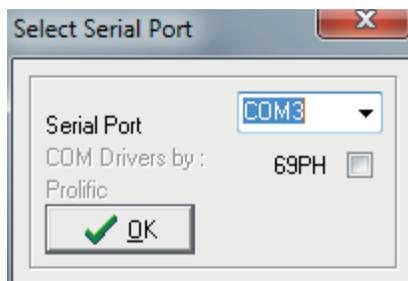
If you later change the USB port to which the device is connected, or if the device is not connected to the PC, the programme reports the error. In this case, select another port if possible. Changing the USB port on the PC also changes the COM port number: this is a feature of Windows drivers, not FWUpdate.
