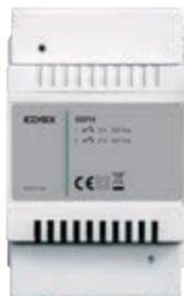
Relay module 69PH is a programmable device equipped with two relays with change-over relay and can be installed on both the Vertical BUS as well as on the Horizontal BUS. If it is installed on the Vertical BUS, it can also be programmed manually with the same modes as relay module 69RH; if on the other hand it is installed on the Horizontal BUS, it can only be programmed using the SaveProg software.
