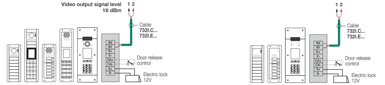
Audio unit with camera input: 41002 and Pixel Up
