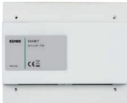
The video selector for 4 cameras 69AM/T allows the connection to the Due Fili Plus system of 4 cameras with CVBS output. Camera selection is cyclical by way of the lock release button or a dedicated push button after the self-start phase. The selector can also be connected to two auxiliary functions F1 and F2.
