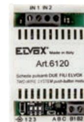
The Interface for 2 push buttons 6120 allows you to use normal push buttons (normally open) to control, via the (vertical) BUS of the Due Fili Plus system, the activation: of the lock on an outdoor station or the landing call of an indoor station or of a relay 69RH/69PH or of functions F1, F2 towards specific entrance panels.
