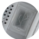
Mini-USB for quick configuration.
