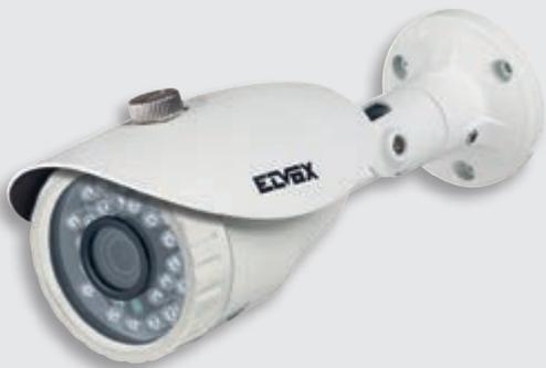
AHD outdoor bullet camera, Full HD 1080p, with 3.6 mm fixed lens and IP66 protection rating. The cam has to be supplied with one of the available power supply units, to select between EU, US, AU, BS standards.
