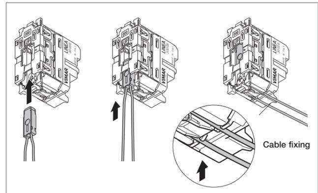
Insertion from the rear of signalling unit
