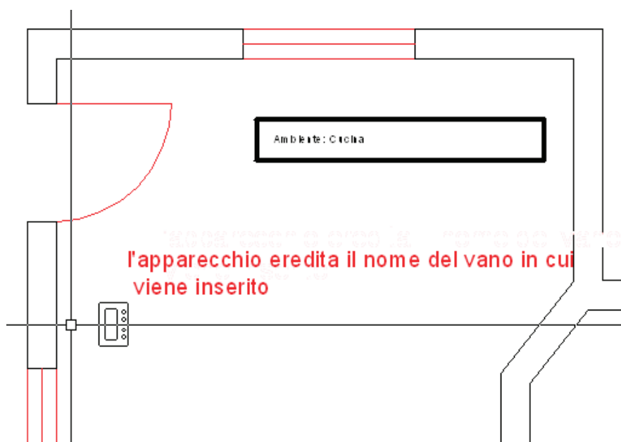
Figure 2: Moving a device to an "identified" compartment
