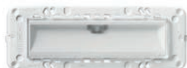
02670.1 With high-efficiency LED, 120-230 V~ 50/60 Hz and built-in 6/7-module frame. Depth: 43 mm
