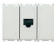
14505.AB Relay module with RJ45 socket outlet for tail call lead with 2 lights + 2 AUX, connection with an 8IN/8OUT module or a Call-way display, 4 24 V NO relay outputs, anti-bacterial treatment - 3 modules. Depth: 29,5 mm
