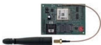
01706 GSM Dual Band GSM/GPRS 900/1800 MHz transmitter/receiver module
