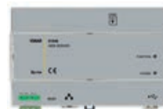
01946 Web server Light for local and remote control of the By-me system via IP, manages up to 64 devices, 8 x 17,5 mm modules
