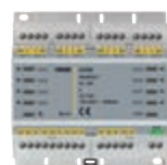
01470 Pre-program 9-input and 8-output module, NO 16 A 120-230 V~ 50/60 Hz relay outputs, light control, roller blind laths positioning and local control functions, 6 x 17,5 mm modules
