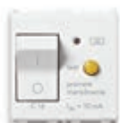
14411.16 C 16, I_{\Delta n} 10 mA breaking capacity 3000 A - 2 modules. Depth: 38 mm
