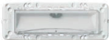
02660.1 With high-efficiency LED, supply voltage 230 V~50/60 Hz, rechargeable Ni-Cd battery, built-in mounting frame for 7-module flush mounting boxes. Depth: 43 mm
