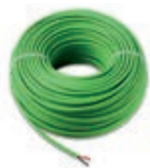
732I.E.100 Due Fili Plus cable for internal/external laying, 2x1 mm 2 twisted conductors, LSZH sheath and insulation, CPR Eca class, operating temperature -25/+70°C, insulation degree 600/1000 V, suitable for laying underground in dry ducting or channels with efficient drainage (max. 24 hrs wet), not suitable for laying directly underground, suitable for I category cables (U0 = 400 V), green - 100 m bundle
