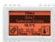
21509.B For control and configuration, touch display, temperature sensor input, with V51923 frame for DIN (60715 TH35) rail installation - 3 modules. Supplied with RJ45 socket connector and V51921 frame. Depth: 37 mm
