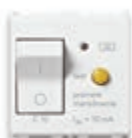
14411.10 C 10, I_{\Delta n} 10 mA breaking capacity 3000 A - 2 modules. Depth: 38 mm
