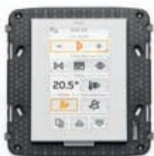
21848.1.B Color touch screen, 4,3", Full Flat, for the control, 1 temperature sensor input, with built-in mounting frame for installation in 8-module mounting box. Depth: 40 mm
