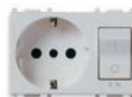
14276.SL 16 A P30 250 V~, 1P+N C 16 - 3 modules. Depth: 38,8 mm
