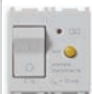
14411.16.SL C 16, I_{\Delta n} 10 mA breaking capacity 3000 A - 2 modules. Depth: 38 mm
