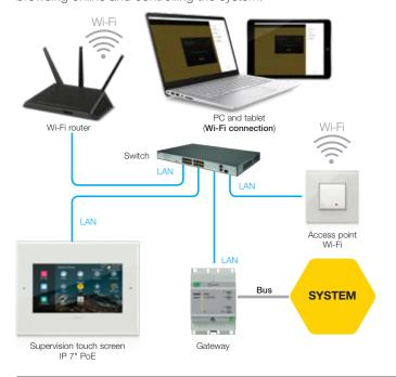
**LAN.** The connection via the Ethernet cable is convenient in case of maintenance on site or commissioning of the system without By-me Plus (which requires the listing of each individual Bus device).
