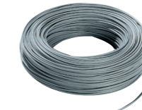
0002.163.E Video system cable, 2x0.75 mm 2 + 75 ohm coaxial cable, with PVC sheath, CPR Eca class, suitable for installation with Category I power cables (U0 = 400 V), grey - 200 m spool
