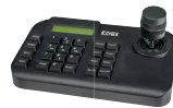
46916.005 Control keypad for Speed Dome cameras, with 3-axis Pelco D, Pelco P Protocol, standard 12 Vdc 2 A power supply unit. Dimensions: 220x130x90 mm
