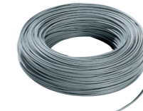
0002.063.E Video system cable, 2x0.35 mm 2 + 75 ohm coaxial cable, with PVC sheath, CPR Eca class, suitable for installation with Category I power cables (U0 = 400 V), grey - 200 m spool
