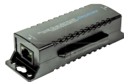
46264.001.01 IEEE802.3af/at standard PoE 10/100 Ethernet Extender, up to 100 m connection, max 3 devices per section
