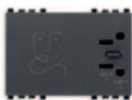
20290 230 V~ 50-60 Hz, with 20 VA isolating transformer, 230 V~ and 120 V~ outputs - 3 modules
