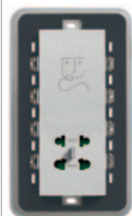
● 20291.N 6 230 V~ 50-60 Hz, with 20 VA isolating transformer, 230 V~ and 120 V~ outputs
