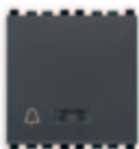
20183 For emergency call, 2 NO 5 A 250 V~, 12 V~/12-24 V d.c. (SELV) - 2 modules
