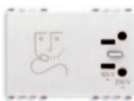
20290.B 230 V~ 50-60 Hz, with 20 VA isolating transformer, 230 V~ and 120 V~ outputs - 3 modules
