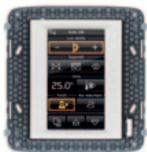
20848.B Color touch screen, 4,3", for the control, with built-in mounting frame for installation in 8-module mounting box
