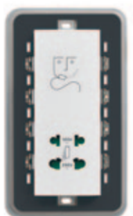
● 20291.B 6 230 V~ 50-60 Hz, with 20 VA isolating transformer, 230 V~ and 120 V~ outputs
