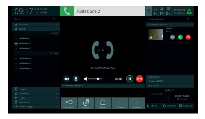
Incoming calls from Users show the name, the same as in the Contacts List section, the ID address and the commands for starting and ending communication.
