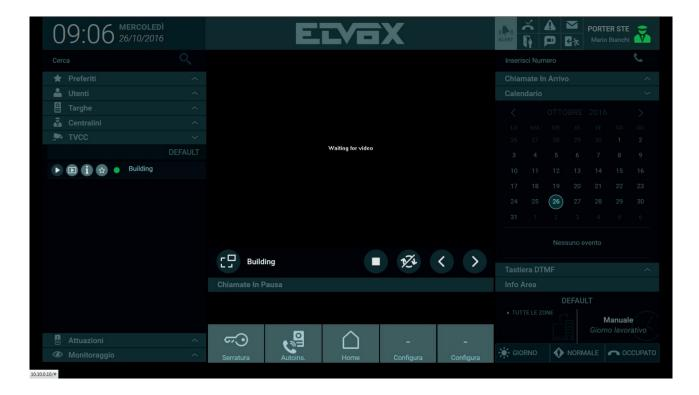
You can also activate self-start of the camera by pressing the button, although the captured images are displayed in a smaller pane on the right side of the home page.
