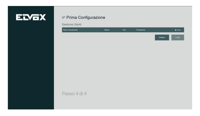
Press the CREATE button to display the screen with text fields for setting the credentials of new users.
