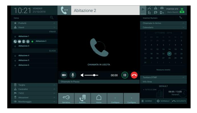
When the call is made, the message "Outgoing Call" appears in the Display Area and the displayed contact name is displayed in the Information Area above.
