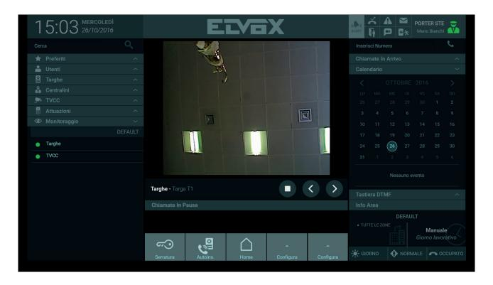
Press the button in the command bar to view footage from outdoor entrance panels or CCTV cameras in the playlist one by one.
