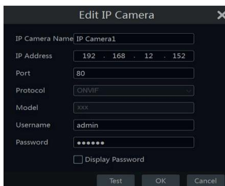
Click to edit the added camera as shown on the above right. Input the new camera name, IP address, port, username and the password of the camera. You can click "Test" to test the effectiveness of the input information. Click "OK" to save the settings. You can change the IP camera name only when the added camera is online. Click "Next" to continue.
