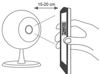
A QR code will be displayed on your smartphone, turn the screen on your phone to face the camera at a distance of between 15 - 20 cm from the lens, a tone will be emitted after a few seconds, tap on **"Tone Emitted"** (refer to the images below).
