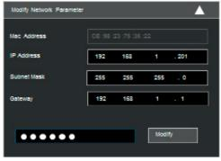
Modify the IP address. The default IP address of this camera is 192.168.226.201. Click the information of the camera listed in the above table to show the network information on the right hand. Modify the IP address and gateway of the camera and make sure its network address is in the same local network segment as the computer's. Please modify the IP address of your device according to the practical situation.
