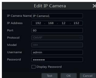
Click to edit the added camera. Input the new camera name, IP address, port, username and the password of the camera. You can click "Test" to test the effectiveness of the input information. Click "OK" to save the settings. You can change the IP camera name only when the added camera is online. Click "Next" to continue.
