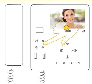
Press % to increase the brightness and % to reduce it. A beep is emitted on reaching the maximum or minimum level.
