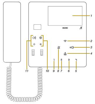
**N.B.**: with the handset replaced, the keys send the control concurrently with the sound feedback, whilst with the handset raised, the control is activated when the key is released.
