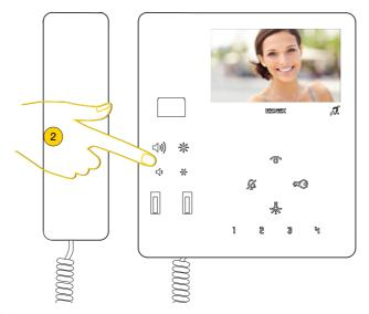
2. Press (J)) to increase the audio level and (J) to reduce it. A beep is emitted on reaching the maximum or minimum level.
