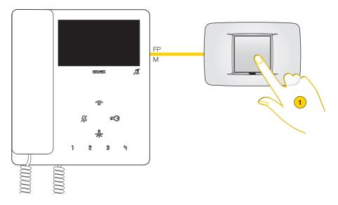
1. Press the push button to send an alert notification
