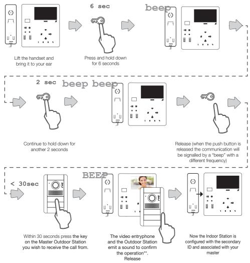
\*N.B.: this procedure applies for entrance panels with push buttons and may vary according to the Outdoor Station used. For Outdoor Stations with a keypad and display, type in the ID code of the master and confirm with the call key.
