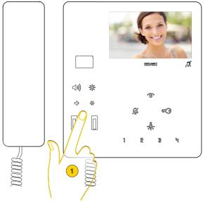
1. During a communication, press the keys positioned under the handset, to adjust the audio/video parameters.
