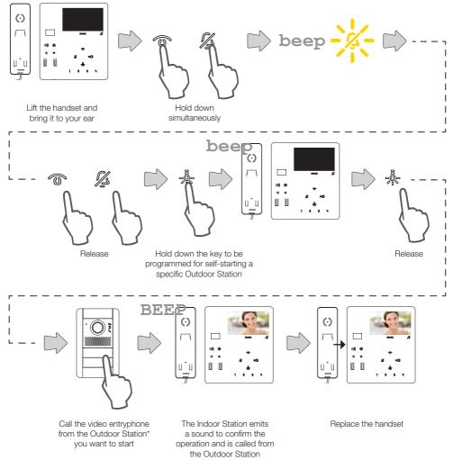
\*N.B.: this procedure applies for entrance panels with push buttons and may vary according to the Outdoor Station used. For Outdoor Stations with a keypad and display, type in the ID code and confirm with the call key
