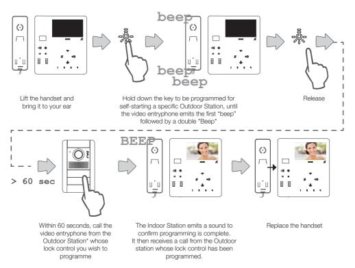
\*N.B.: this procedure applies for entrance panels with push buttons and may vary according to the Outdoor Station used. For Outdoor Stations with a keypad and display, type in the ID code and confirm with the call key
