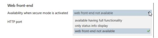
If the front-end Web is set to "status display only", the remote control functions (programming mode activation, tunnelling setting) and the updating function are disabled. Information read only is available.
