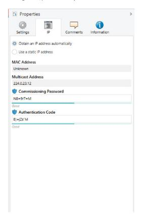
If you select the "Use a static IP address" option, you can manually set the IP address, the subnet and default gateway address.
