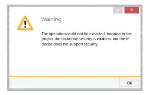
**N.B.** If reset devices are present, the default physical address 15.15.255 is not read by the ETS diagnostics because it is transmitted unencrypted when the Backbone is Secure. Once the Backbone secure is activated, the configuration status of the various Secure devices will show as not up to date and so the application programmes will have to be downloaded again.
