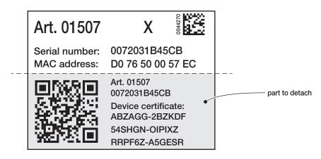
After adding the device Certificate to the dedicated list in ETS, keep the removed part of the label in a safe place. The list of device Certificates must only include certificates of KNX Secure devices used for ETS projects. ETS will automatically use the correct certificates for device programming.
