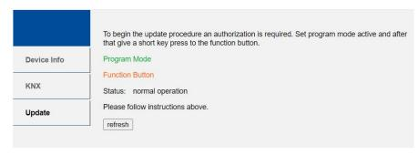
Step 3: After activating programming mode, briefly press the function button. Then press the "refresh" button.
