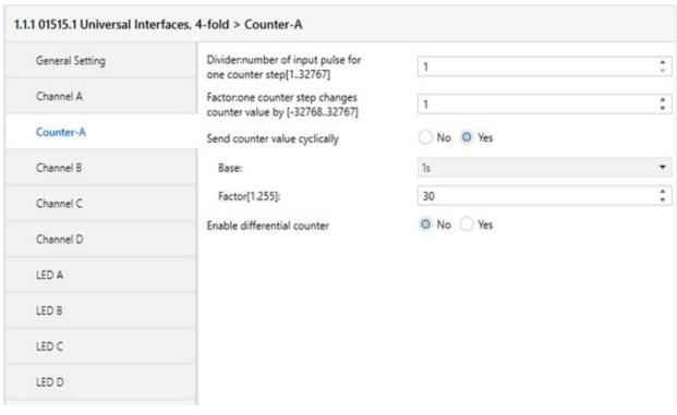
Fig. 15 - Parameter window "Counter-X"
