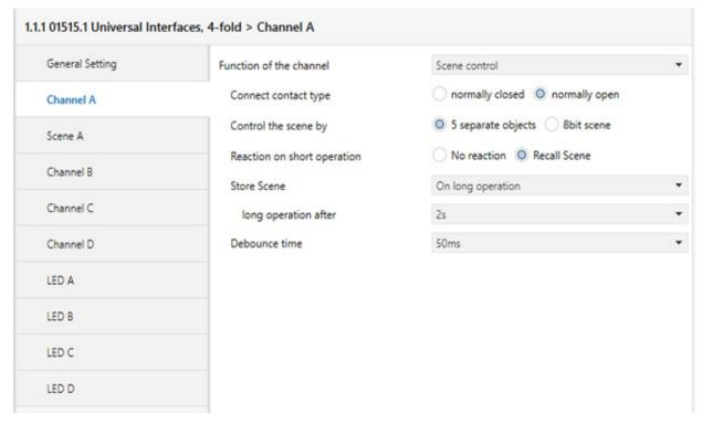
Fig. 10 - Parameter window "Scene control, X"
