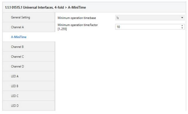
Fig. 5 - Parameter window "X-Mini Time"
