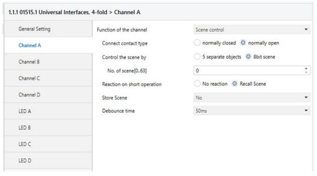
Fig. 11 - Parameter window "8 bit scene"
