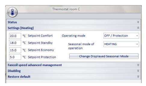
Through the "Settings" panel you can change the main parameters of operation of the Well-Contact system thermostat. Below is the description of the parameters set in this panel:
