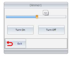
The command is sent to the dimmers associated with the function master at the time of action on the virtual Dimmer object (pressing the buttons or releasing the slider cursor). The commands are not stored in the software database and there are no default values when the widget is opened (the cursor position is always 0%).
