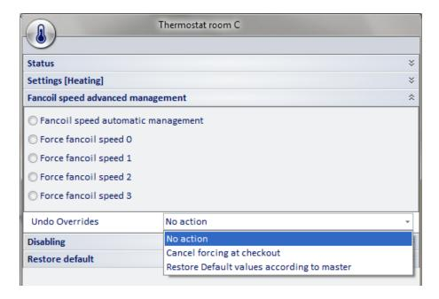
Through the "Fancoil speed advanced management" panel you can manually change the speed of the fancoil. The following commands are available:
