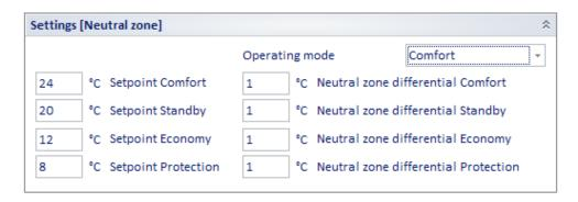
In the "neutral zone" control mode of a 4-pipe system, after setting the setpoint for the heating and cooling operating modes, the thermostat will automatically switch to heating or cooling according to the setpoint and the measured temperature.
