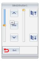
The command is sent to the shutter actuators associated with the function master at the time of action on the virtual Rolling Shutter object (pressing the buttons or releasing the slider cursor). The commands are not stored in the software database and there are no default values when the widget is opened (the cursor positions are always 0%).
