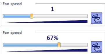
The icon on the right of the slider provides further information about the automatic or manual management of the fan coil speed.
