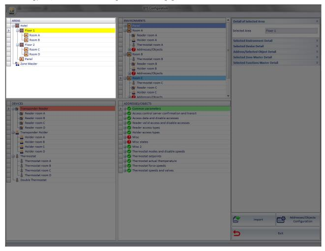
In the "AREAS" section the topology of the KNX automation system is represented through a tree-like structure. In the previous picture, the system topology is represented using the following items (which differ for the hierarchical levels):
