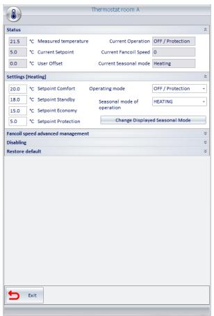
Note. The previous picture shows the main features of the thermostat, while the remaining can be displayed "expanding" their "panels." Some functions are not present in all types of Vimar KNX thermostats: Well-Contact Suite will display the functions of the specific type of thermostat that have been appropriately configured via the KNX ETS.
