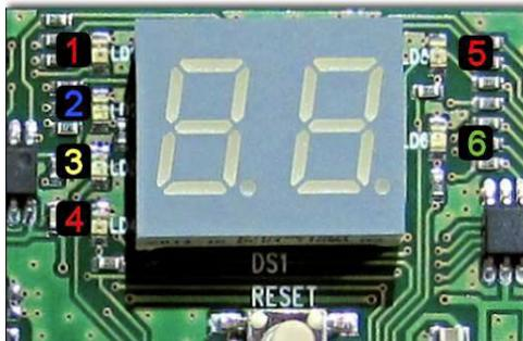
During normal operation, the LEDs are off and the display cyclically shows the various associated devices. In the event of an alarm and/or malfunctioning of a device, the interface will immediately display the number of the relevant device and one of the LEDs on the left of the display will light up to indicate its cause. If multiple devices were simultaneously in an alarm and/or fault status, the interface display would cycle through the states of the various devices concerned.
