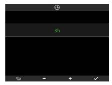
Using the softkeys  ${\bf B}$  and  ${\bf C}$  set the duration of time in which the thermostat will work on reduction and at the end of which it will revert to the previous operating mode .
