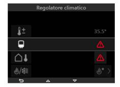
If there is a malfunction of the system, or damage to the probes connected to the climate controller, the By-me automation module will display the icon .
