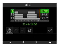
• Selecting the licon displays the screen used to change the value of the temperature levels T1, T2 and T3.
