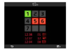
In the event of an alarm, the alarms list (up to a maximum of three) is displayed under the partitions grid and identifies the alarm zone, the time and the icon associated with the type of alarm.
