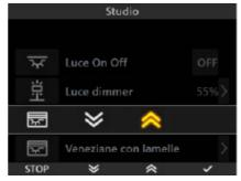
Tapping the softkey **A** stops opening/closing the shutter in the desired position.
