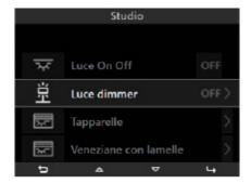
In the case of an adjustable lighting point (dimmerable), on tapping the softkey **D**, the display will show the control mode that allows switching on/off and dimming the lighting point.
