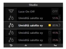
If the displayed variable is relative humidity and when envisaged by the system, you can set a setpoint on exceeding which a special alarm will be displayed, and activated when needed.
