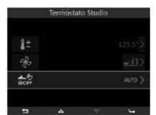
Tapping the softkey **D** displays the menu that allows you to select the operating mode of the HVAC zone.
