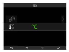
Using the softkeys **B** and **C** select the unit of measurement in which the temperature of the various rooms of the system will be displayed.
