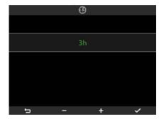
Using the softkeys **B** and **C** set the interval of time in which the thermostat will be off and at the end of which it will revert to the previous operating mode.
