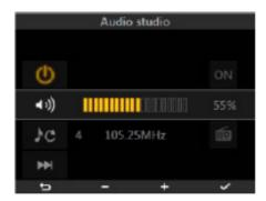
Using the softkeys **B** and **C** set the volume whose level will be highlighted by the horizontal bar and by the numerical percentage shown on the right:
