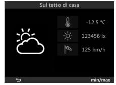
The arrows next to the temperature and wind speed take you to a page showing the extreme values recorded. Resetting these values can be done manually (with the specific button) or automatically at midnight every day. The choice between the two reset modes is made during installation.
