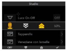
Note that, on the right side of the adjustment icons, the display shows the percentage of brightness (if the lighting point is on) or the word OFF (if the lighting point is off).
