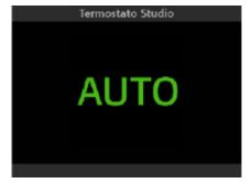
This menu lets you change the HVAC programmes for automatically controlling the heating and air-conditioning previously configured on the control panel.
