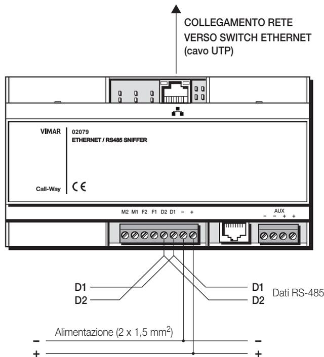
**Ethernet/RS485 interface, installation on DIN rail (60715 TH35), occupies 9 modules size 17.5 mm.**
