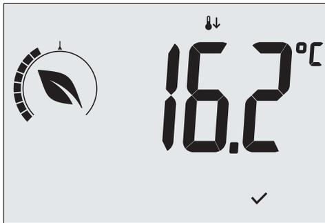
Fig. 10: Input in Nighttime Reduction mode showing the reduction set point
