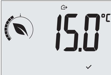
Fig. 8: Input in away mode showing the away temperature
