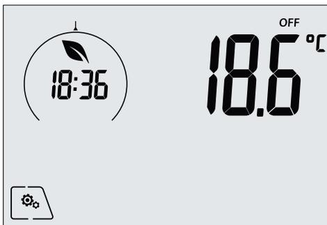
*Fig. 4: Typical screen for OFF mode*
