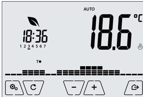
Fig. 11: Typical screen for Auto mode
