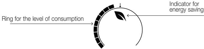
Fig. 5: Typical view of ecometer mode
