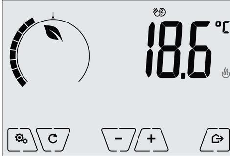
Fig. 12: Input screen in Timed Manual mode
