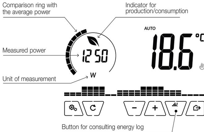
Fig. 6: Typical screen for consulting the energy probe
