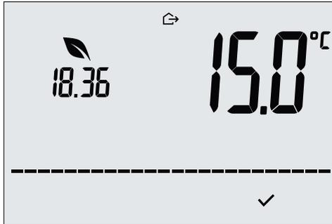
Fig. 14: Input in away mode showing the away temperature
