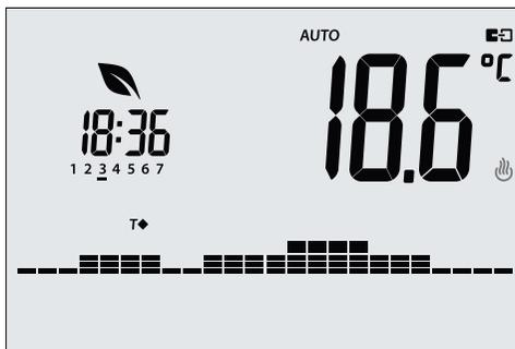
Fig. 18: Typical screen in Remote auto mode
