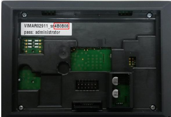
Fig. 6: Back of the timer-thermostat 02911
