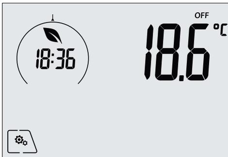
Fig. 17: Typical screen for OFF mode
