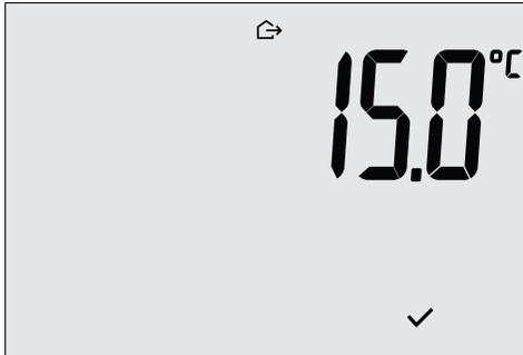
Fig. 23: Input in away mode showing the away temperature
