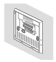
Caution: Tighten the wall bracket screws, applying sufficient torque without exaggerating, in order to avoid warping it.
