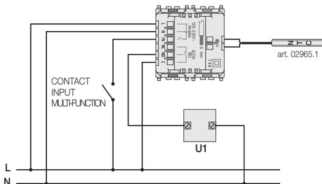
Fig. 1: Connection of relay and multi-function input
