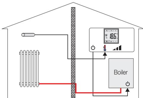
02965.1 used for limiting the temperature of underfloor heating
