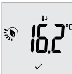
Fig. 11: Input in Nighttime reduction mode showing the reduction set point
