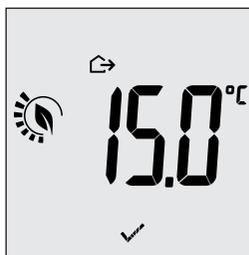
Fig. 9: Input in away mode showing the away temperature
