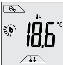
Fig. 12: Nighttime reduction mode
