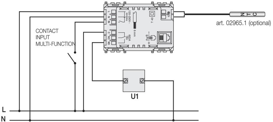
Fig. 1: Connecting the multi-function input
