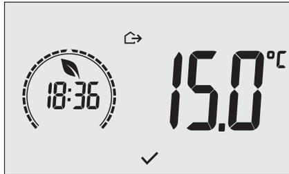
Fig. 19: Input in away mode showing the away temperature
