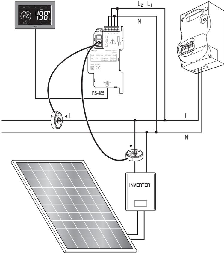
Fig. 6: Measurement of differentiable consumption and generation with a photovoltaic system installed. Note the direction of installation of the current probe S2: in cases of generation via a photovoltaic panel, the probe will record a **NEGATIVE** value that corresponds to energy generation (as opposed to consumption).
