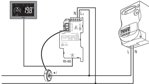
Fig. 3: Basic configuration for measuring absorption in the environment
