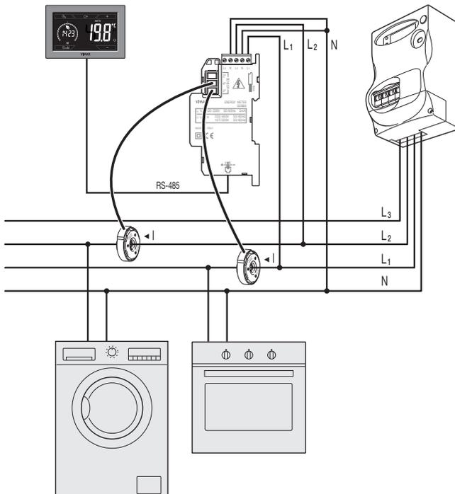
Fig. 4: Measurement of the total consumption of a system with single-phase loads distributed over multiple phases.
