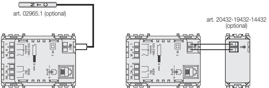
Fig. 2: Connecting the external temperature probe
