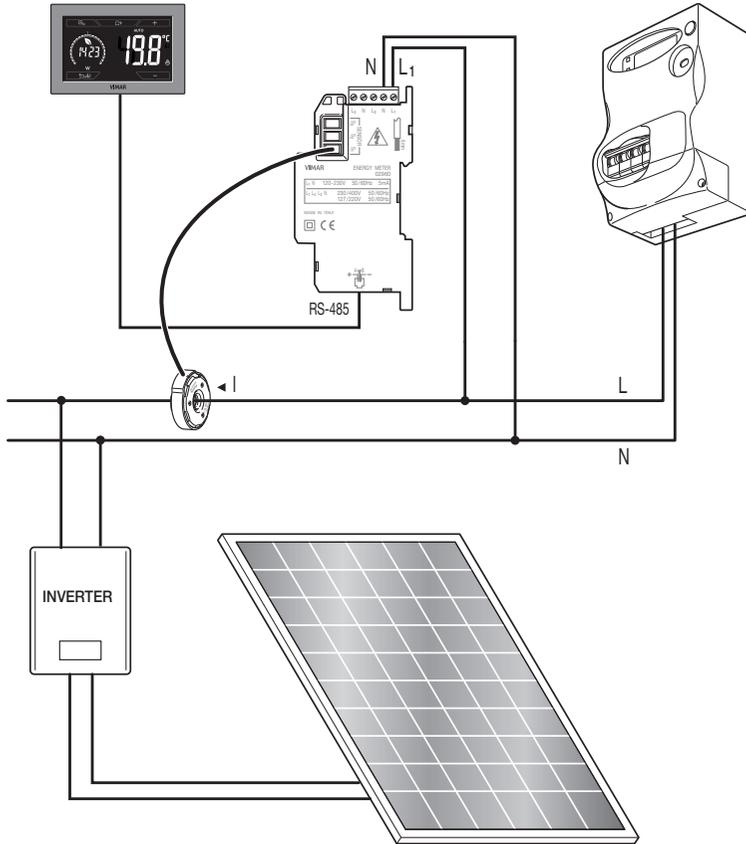
Fig. 5: Measurement of net consumption or generation with a photovoltaic system installed. In cases of generation via a photovoltaic panel (fed into the national grid), the probe will record a NEGATIVE value which corresponds to energy generation (the opposite of consumption).
