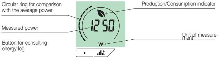
Fig. 11: Typical screen for consulting the energy probe
