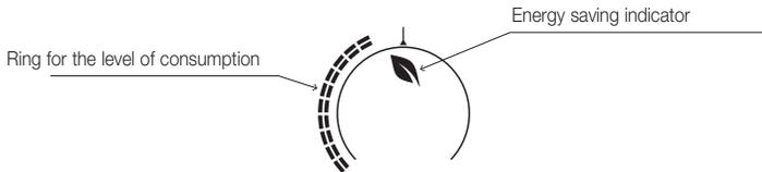
Fig. 10: Typical view of ecometer mode
