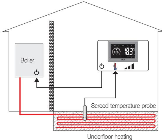
**IMPORTANT:** During installation, take care not to damage the insulation of the probe while laying the screed. Perform the installation in such a way that the probe is accessible for any maintenance work.
