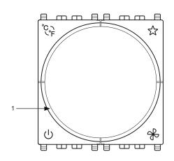
All lit amber\* = thermostat in heating mode and relay active
