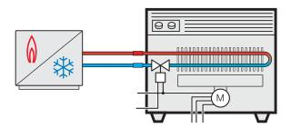
Installation of 4-pipe fan coil solenoid valve
