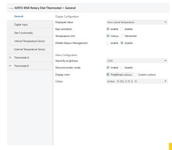
Monochrome mode to blend in the colours of the thermostat with those of the wiring series: Default colours (for instance Red, Amber, etc.)
