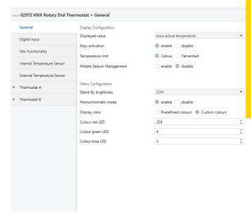
Monochrome mode to blend in the colours of the thermostat with those of the wiring series: Customised colour (RGB setting)
