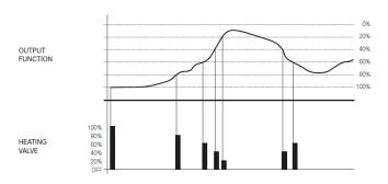
The parameters of the proportional and integral coefficients Kp and Ki are set using the ETS software: the proportional coefficient Kp for heating corresponds to the "Heating Proportional Value" parameter while the coefficient for cooling is set using the "Cooling Proportional Value" parameter. The integral time Ti is set with the "Heating Integral Value" and "Cooling Integral Value" parameters for heating and cooling, respectively.
