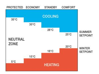
CAUTION: When the thermostat is in Neutral Zone mode, the breadth of this must be progressively increasing for the different operating modes of Comfort (minimum neutral zone breadth), Standby, Energy Saving and Protected. This setting made with ETS ensures that, when the thermostat changes operating mode, the active setpoint is always at a suitable value and the thermostat does not start cooling if it was heating before or vice versa, causing considerable energy consumption.
