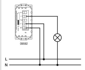
Example of a light circuit with push buttons and relays in a new system.
