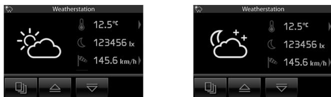
The arrows next to the temperature and wind speed take you to a page showing the extreme values recorded. Resetting these values can be done manually (with the specific button) or automatically at midnight every day. The choice between the two reset modes is made during installation.
