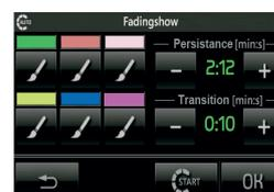
The function of Fading-Show allows to set a cyclical sequence of colors (up to a maximum of 6) for color changes and the play of light in the environments where the lamps are installed RGB.
