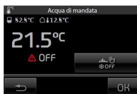
If there is a malfunction of the system, or damage to the probes connected to the climate controller, the touch screen will display the icon .
