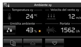
If the displayed variable is relative humidity and when envisaged by the system, you can set a setpoint on exceeding which a special alarm will be displayed, and activated when needed.
