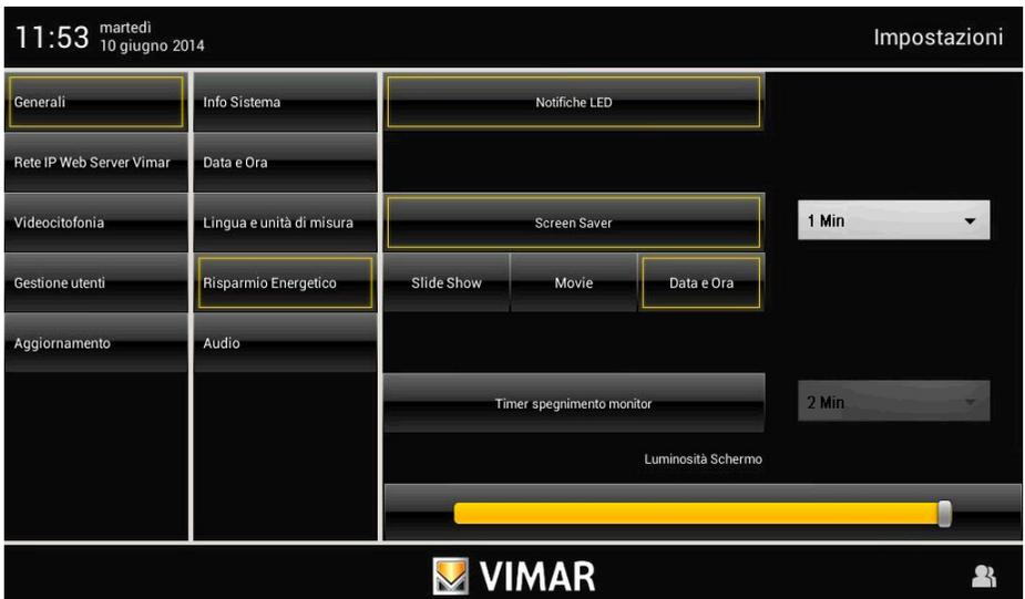
By tapping the dedicated icons you can activate switching off the display and the screen saver, setting its type and its time out.
