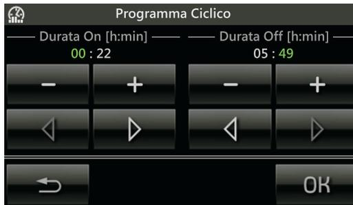
● Impostare la durata di ON (h:min) mediante
