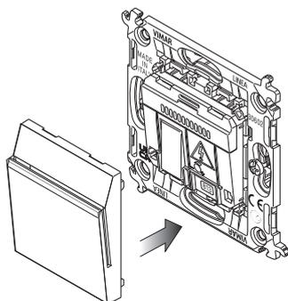
4 - Agganciare la placca al supporto • Hook the cover plate onto the mounting frame
