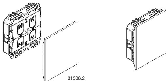
INSTALLAZIONE SU SCATOLA DA INCASSO • INSTALLATION ON FLUSH MOUNTING BOX • INSTALLATION EN BOÎTE D'ENCASTREMENT
