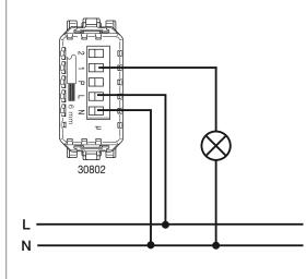
Example of a light circuit with push buttons and relays in a new system.
