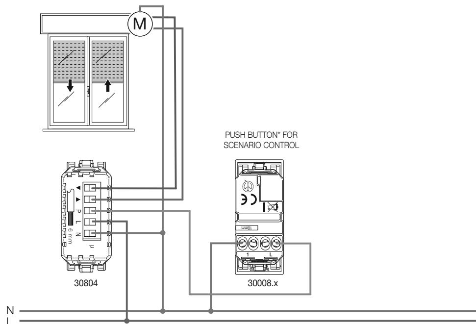
\* Do not use the signalling unit 00931. The push button can only be used in the case of operation in Bluetooth technology.
