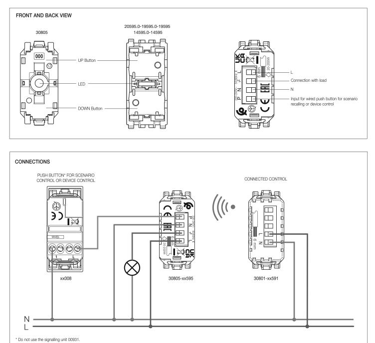
N.B. Graphic representation of the Linea series. Position of terminals, wiring and functions also identical for Eikon, Arké and Plana.
