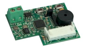
433RAD.T Plug-in 2-channel receiver 12/24 V 433 MHz
