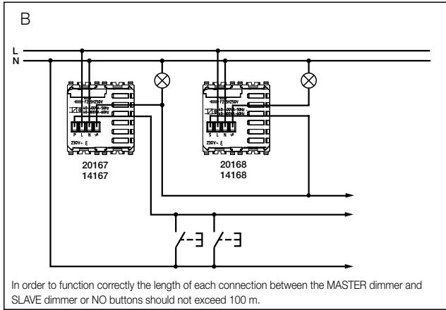
In order to function correctly the length of each connection between the MASTER dimmer and SLAVE dimmer or NO buttons should not exceed 100 m.
