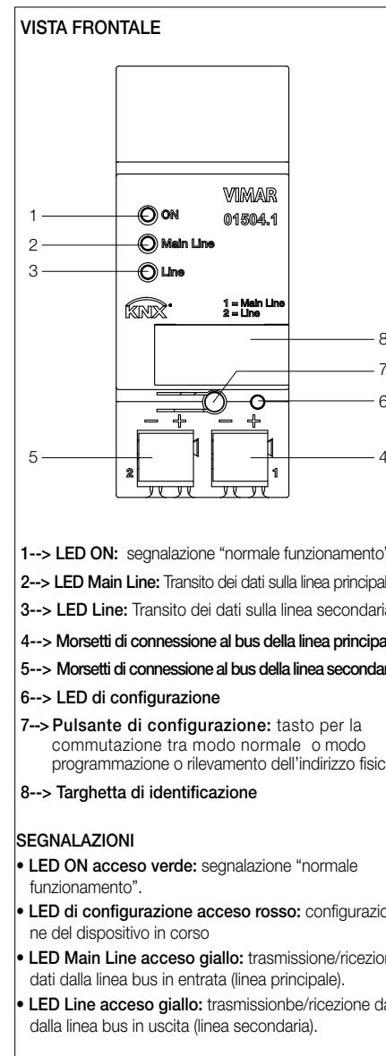
Line/field coupler, KNX standard, installation on DIN rail (60715 TH35), occupies 2 modules of 17.5 mm.
