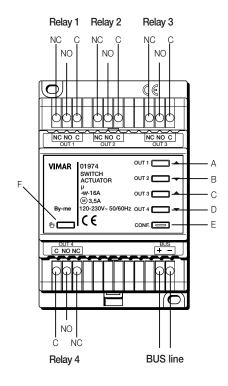
A: LED and button to actuate relay 1
