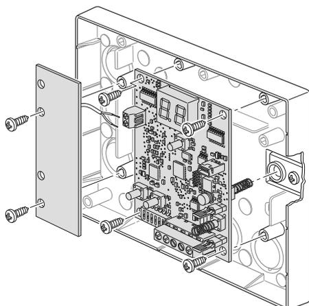
4. Close the enclosure, fixing the cover to the box.
