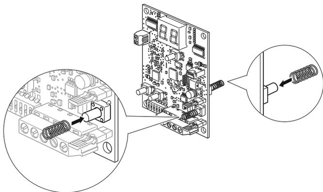
3. Install the interface 01729 complete with springs in the box.
