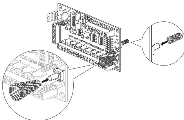
3. Install the module 01704 complete with springs in the box 01714.
