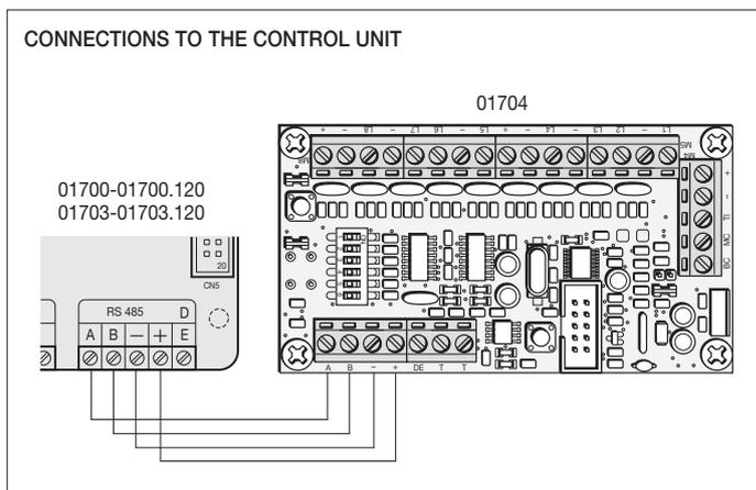
Caution: The maximum number of expansion modules that can be installed depends on the type of control unit used.
