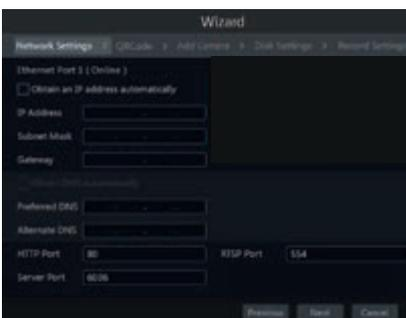
**3- Network Settings.** Check "Obtain an IP address automatically" and "Obtain DNS automatically" to get the IP address and DNS automatically, or manually input IP address, subnet mask, gateway, preferred DNS and alternate DNS. Input the HTTP port, RTSP port and Server port. Click "Next" to continue.
