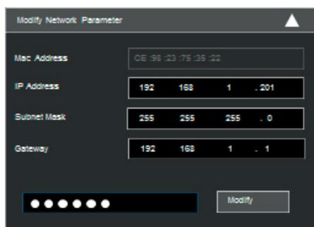
For example, the IP address of your computer is 192.168.1.4. So the IP address of the camera shall be changed to 192.168.1.X.
