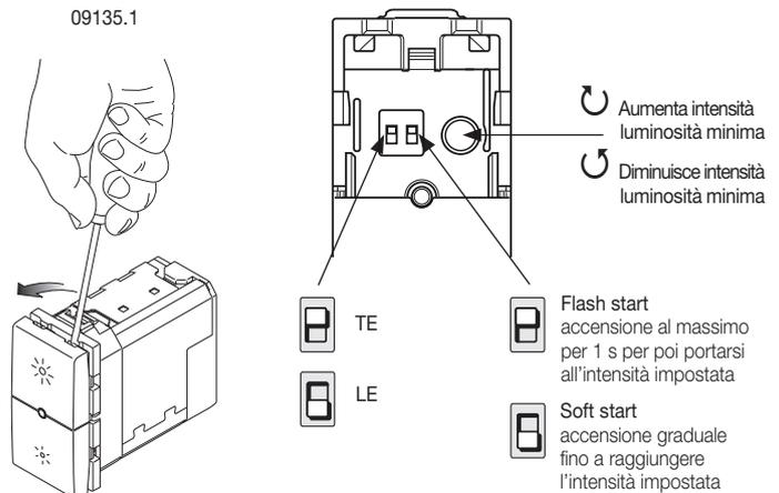
Dimmer 230 V~ 50 Hz for 40-400 W incandescent lamps, 40-300 VA electronic transformers, 10-200 W CFL lamps, 3-200 W LED lamps and LED electronic transformers, ON/OFF control and regulation with built-in push button or from NO peripheral push buttons, MASTER function for 14137, minimum power control, visible in darkness. Not for Iso-set enclosures.
