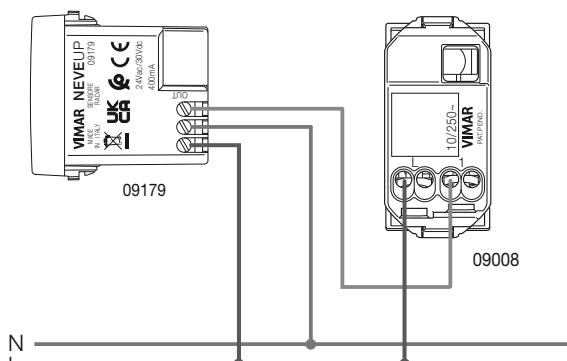
**2. Collegamento a lampada spia • Connection to the pilot lamp**
